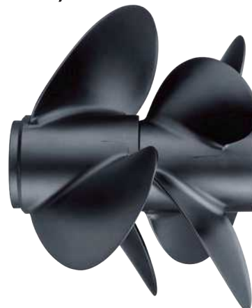
Aluminum / 3 blade front & 4 blade rear / Rubber hub
