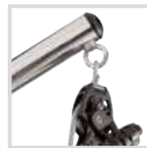
Block fitting Fitting for block winch.
