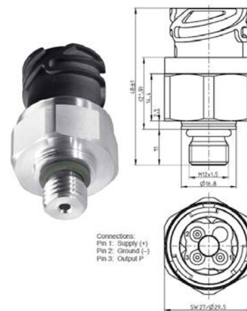
Electronic pressure sensor with voltage output
